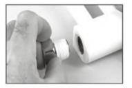
2. Tighten the nut (on the tail thread) using an appropriate tool, usually an Allen key.
