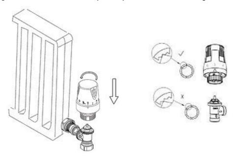
**Please note:** Ensure that the Thermostatic dial is correctly attached as shown in the above right diagram.
